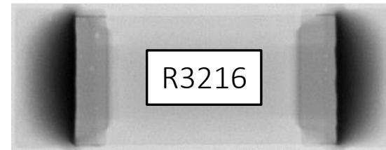
X-ray image after soldering
